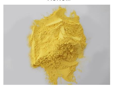
AOROM is an entirely new type of thermoplastic polyimide resin, making full use of its technology. The expansion of the application range of AOROM has been made possible because of its thermoplasticity, which is suitable for injection molding and extrusion, as well as its unparalleled high heat resistance and mechanical and electrical properties.
